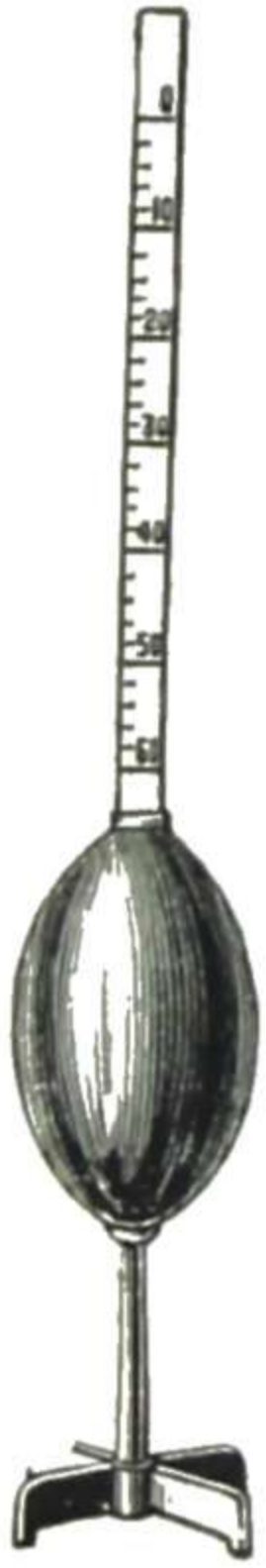
FIG. 89. — URINOMETER, made of metal, and with flanged foot.—The flanges steady it while in the urine, and form a stand when not in use.
