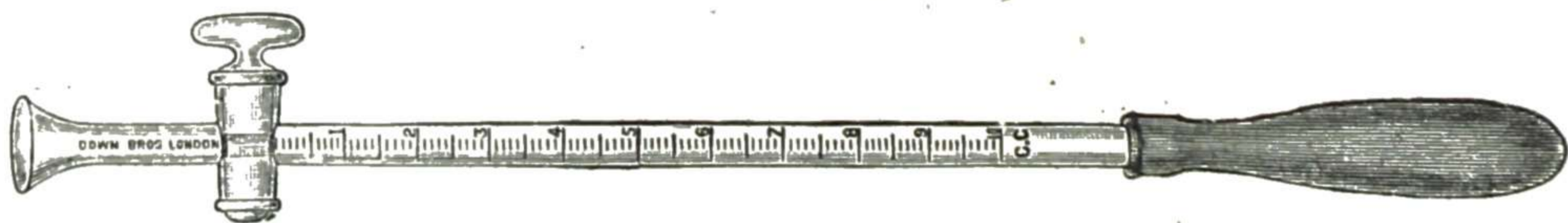
FIG. 91.—AMBARD'S APPARATUS FOR ESTIMATING BLOOD UREA. ( \frac{1}{2} scale.)
